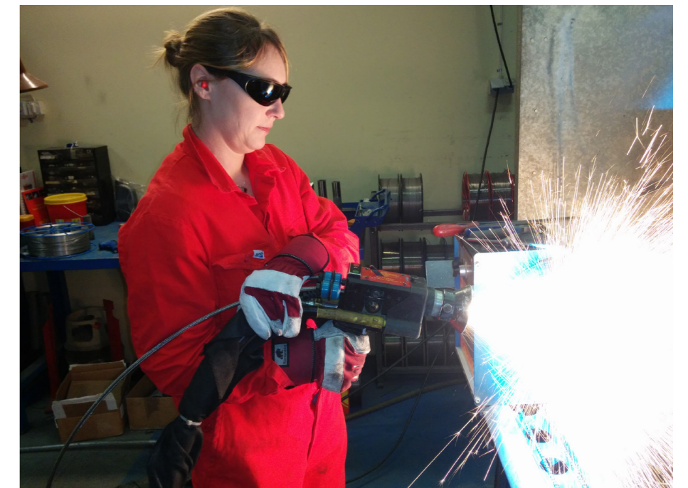
Figure 1 above: Different surface engineering methods that will be explored in the SEAM initiative. Figure 2 below: Thermal spraying as a surfacing process for thick coatings
