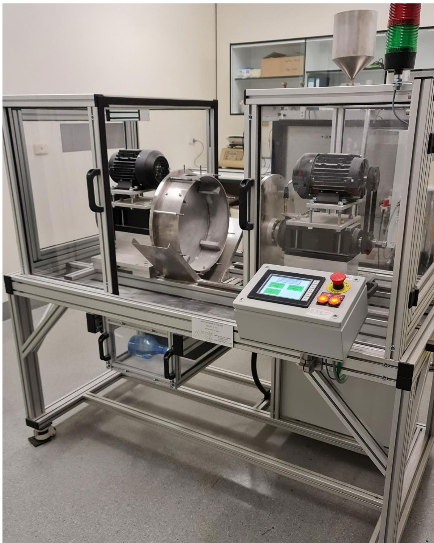
Image: CIAT (Continuous Impact/Abrasion Tester) located at University of South Australia
